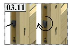
Fasten the doorsill with metal screws on the subframe (03.8). Next, mark the central points of the fastening opening (spingalet) (03.9) and drill holes with a depth of 15 mm (03.10) using an 8 mm drill. If necessary, you can change the direction of the lock tongue (03.11).
